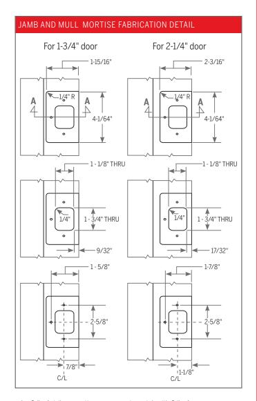
C/L of strike mounting screws are to match with C/L of Lock and door.
