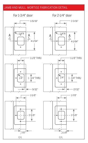
C/L of strike mounting screws are to match with C/L of Lock and door.
