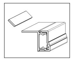
**b.** Cut the brickmould leg along your mark
