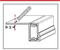
**a.** Measure the same distance cut off of the jamb core onto the leg of the brickmould.
