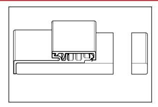
**b.** Rip down the jamb core based on the mark made.
