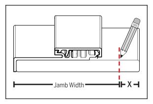
**a.** Determine the jamb width required and mark on the core.
