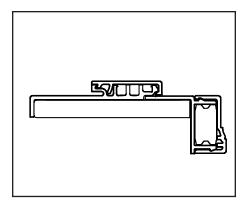
**c.** Check the fit of the cut jamb and brickmould. The brickmould leg should cover any remaining core.
