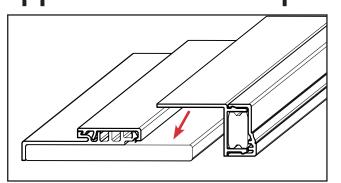
Rippable jambs and brickmould allow you to maintain the prefinished look of the FusionFrame, while still meeting the specifications of your project. The extended leg of the brickmould fits into the slot and covers the exposed portion of the core to protect it.
