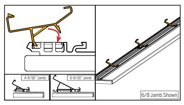
**b.** Install the clips onto jamb by rotating it over the lighter colored ribs. Repeat along the length of the jamb. For 6/8 jambs, you'll need 2-3 clips. For 8/0 jambs, you'll need 3-4.
