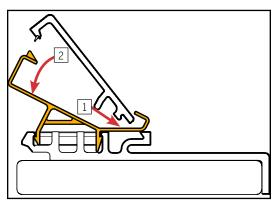
**c.** Slide the interior side of the jamb cover into the clip (1) and rotate the exterior side downwards to snap into place (2).
