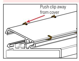
**a.** Push the clip away from the cover, allowing it to rotate out.
