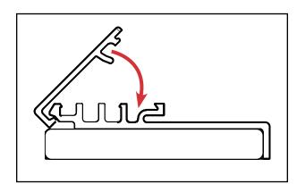
**c.** Install the jamb cover back onto the jamb, once the door unit is installed by rotating the cover over the exterior of the jamb and snapping it on.
