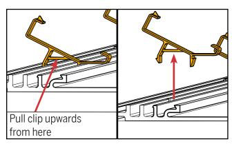
**b.** Use a screwdriver (or your hand) under the horizontal support and pull upwards to disengage the clips.
