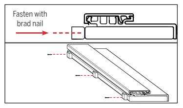
**b.** Using brad nails, fasten the spacers to the top of the jamb, the middle of the jamb and the bottom of the jamb.
