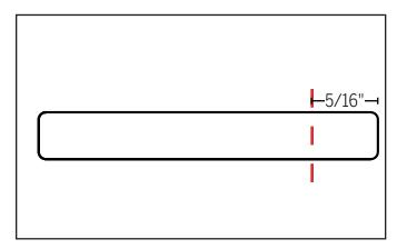
**a.** To make a 4-7/8" jamb out of a 4-9/16" Dedicated Jamb, start by **creating a 5/16" spacer** out of any scrap materials.
