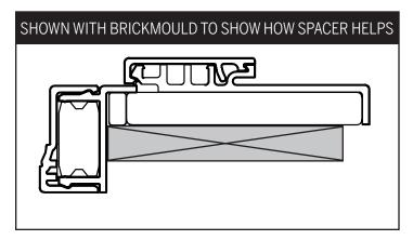
**c.** Align the **end of the spacer** to the **edge of the stud in the rough opening** to properly align the back of the jamb. Install the jamb as directed.
