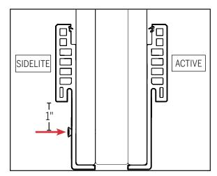
**c.** On the side of the sidelite panel, install screws through the jamb, about 1" off the jamb stop and along the length of the jamb.
