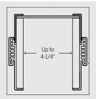
Spread Mulls can be created using two jambs, two L-Shaped Inserts and one Flat Insert.
