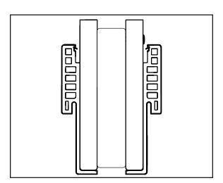
**b.** Fasten a 1" thick wooden block in between the two jambs, using the below notes.
