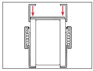
**g.** Insert the two modified L-Shaped Inserts into the brickmould slots to hold the Flat Insert in place.
