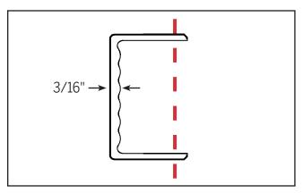
**d.** For the 2.5" U-Shaped Cover to fit properly, cut down the legs. If you are installing the U-Shaped Cover into two dedicated jambs, you will need to cut the legs down 15/16".
