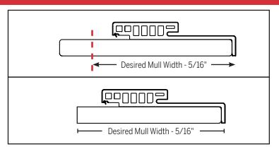
**a.** Cut down the core of the jamb to be 5/16" less than the desired width of the mull assembly. This will account for the thickness of the L-Shaped Inserts and Flat Insert.
