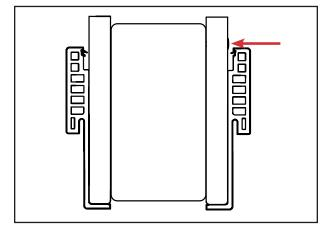
**b.** Fasten a wood block in between the two jambs, using the below notes. The wood block should be the thickness desired minus 1-1/2".
