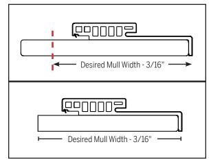
**a.** Cut down the core of the jamb to be 1/8" less than the desired width of the mull assembly.
