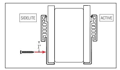
${f c.}$  On the side of the sidelite panel, install screws through the jamb, about 1" off the jamb stop and along the length of the jamb.
