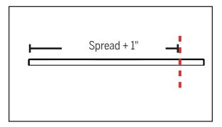
**e.** Cut the width of the Flat Insert to cover the spread of the mull and cut the length to match the desired of the mull assembly.
