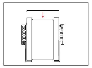
**f.** Align the modified Flat Insert against the exposed core of the two jambs, holding it in place.
