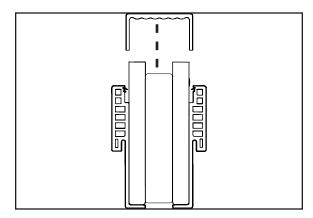
**e.** Install the modified U-Shaped Cover into the brickmould slots on the jambs.
