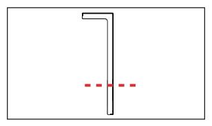
**d.** Cut down the longer side of the (2) L-Shaped Inserts the same amount as the core is cut down.
