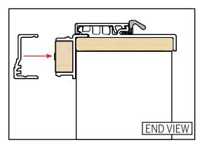
c. Reinstall the brickmould cover.
