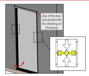
Keep the top of the door unit plumb with the sheeting on the house and adjust the bottom in and out using the bubble level to plumb the rest of the unit in the rough opening.
