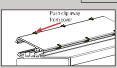
Method 1: If Jamb Cover Clips are installed, push down on the exterior side of the clip to disengage and pull off the clip.
