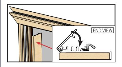
**a.** Rotate the cover over the jamb (starting from the outside) and snap it downward along the length of the jamb.
