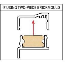
**b**. To simplify the brickmould install later, remove the covers and set aside. If the header brickmould was left in the unit, be sure to remove the cover and set aside.
