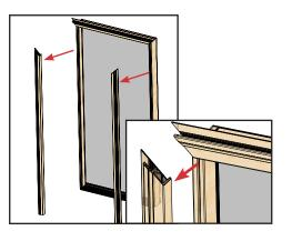
**a.** If attached, remove the brickmould assembly from the prehung door unit, and set aside.
