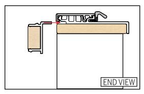
**a.** Insert the leg of the brickmould into the groove of the jamb.
