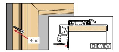
**b.** Install 4-5 fasteners, evenly spaced, through the nailing flange to secure the brickmould to the sheathing.
