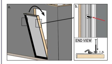
**a.** Position the door unit into the rough opening.
