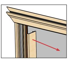
**c.** Remove the jamb covers using one of the methods outlined below.
