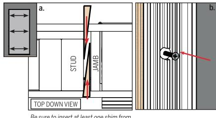
Be sure to insert at least one shim from each side (interior and exterior) to keep the jamb from twisting. **a.** Shim the door unit between the jamb and stud to keep it square and plumb, starting behind the upper prenotched location.
