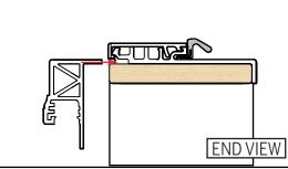
**a.** Insert the leg of the brickmould into the groove of the jamb.
