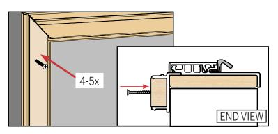
**b.** Install 4-5 fasteners, evenly spaced, through the wood core of the brickmould into the sheathing.
