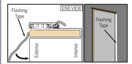
Install flashing tape from the wood edge of the jamb, away from the door opening.
