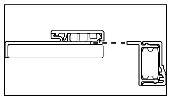
Insert brickmould into the slot along the exterior of the jamb.
