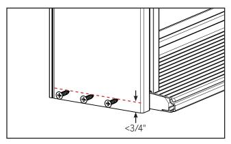
Keep the screw pattern in a straight line within 3/4" from the end of the jamb when assembling to the sill to avoid interfering with the sill system.
