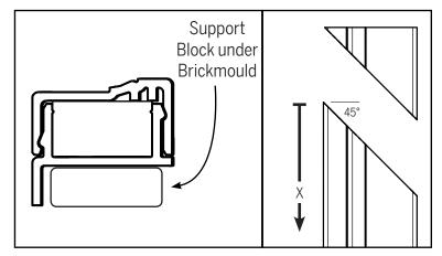
Position a piece of wood under the brickmould for support and cut the brickmould to length. Keeping the support under the brickmould, make a 45° miter cut from the exterior edge to the interior.
