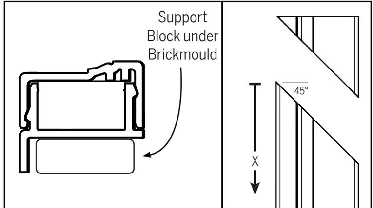
Position a piece of wood under the brickmould for support and cut the brickmould to length. Keeping the support under the brickmould, make a 45° miter cut from the exterior edge to the interior.
