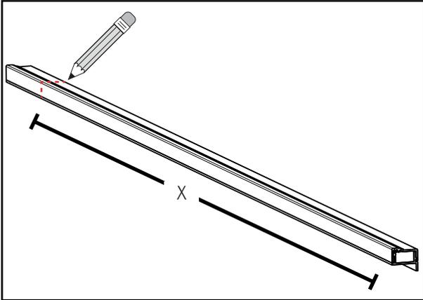
Measure the exterior of the brickmould and mark.
