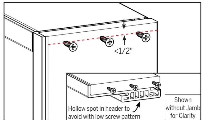
Keep the screw pattern in a straight line within 1/2" from the end of the jamb when assembling to the header to avoid hitting the hollow spots in the jambs.
