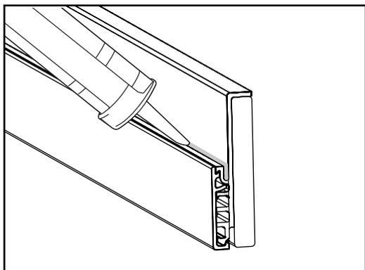
When caulking for the inactive panel, aim for the caulk to go towards the weatherstrip kerf. This will prevent caulk from interfering with the jamb cover.
