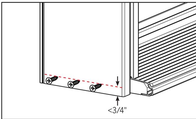
Keep the screw pattern in a straight line within 3/4" from the end of the jamb when assembling to the sill to avoid interfering with the sill system.
