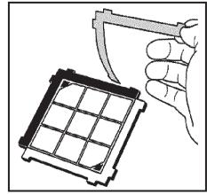
Peel protective paper off of the backside (instruction side) of the applicator in the location marked "CORNER A" to reveal the adhesive underneath.
