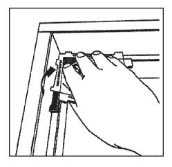
c. Grip the applicator firmly and peel back from the framework to reveal the gasket strip.
