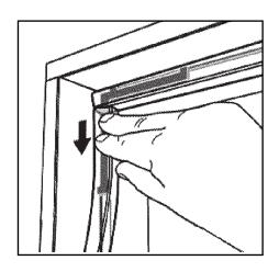
Insert the head jamb and side jamb weatherstrip as normal. Repeat process for other corner.
