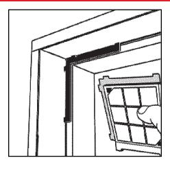
d. The gasket strips should now be exposed and affixed to the upper corners of the frame.
