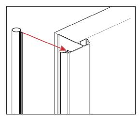
Starting at the top, work your way down the security flange, firmly pressing the weatherstrip into the kerf slot.
