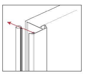
b. Remove the old weatherstrip, using the needle nose pliers if necessary. At this point, clean the kerf slot thoroughly before placing new weatherstrip.
