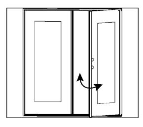
Open and close the door to confirm that the weatherstrip does not interfere with opening and closing the door.
