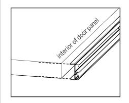
a. Align one end of the door bottom with the door panel edge on the side that will be facing the strike plate.
