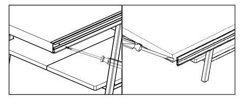
a. Remove the old door bottom from the door panel by removing the screws, if it was a screw-on door bottom. If the door bottom was stapleon, you may need to pry it off with a flathead screwdriver.
