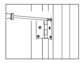
a. Open the door and locate the hinges. Using a Phillips screwdriver or drill remove the screws from the hinge plate on the jamb.
