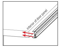
b. Using hand pressure, press the door bottom flush against the bottom of the door panel. Make sure the door bottom is flush down the length of the panel square at the ends.
