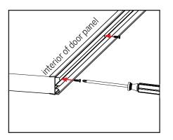
c. Secure the door bottom to the door panel with the screws provided. Position the screws in the center of the slots.
