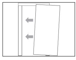
a. Realign the door panel with the hinges in the frame.
