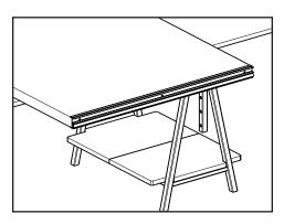
b. Repeat on other hinges. When door is loose from frame, carry it to a flat workspace where the panel can be laid horizontally.
