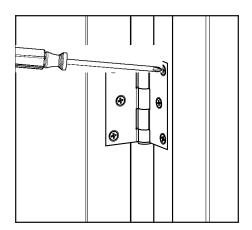
a. Open the door and locate the hinges. Using a Phillips screwdriver or drill, remove the screws from the hinge plate on the jamb.
