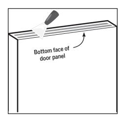
b. Remove any old residue or staples from the door panel's bottom face, using a putty knife or similar tool.
