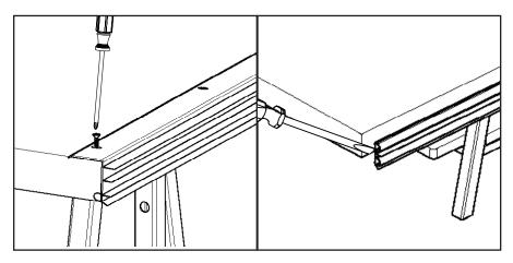
a. Remove the old door bottom from the door panel by removing the screws, if it was a screw-on door bottom. If the door bottom was staple-on, you may need to pry it off with a flathead screwdriver.
