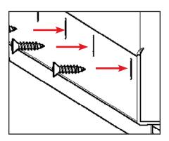
c. Close the door panel and check that the door bottom meets the sill cap to provide proper weathersealing. Once the positioning is set, secure the door bottom to the door with the screws provided. Position screws in the center of the slots.
