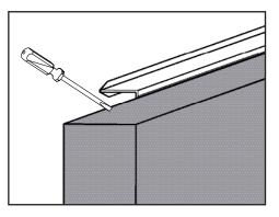
a. Remove the old DoorTop from the door panel. Use a flathead screwdriver to pry the end of the DoorTop up.
