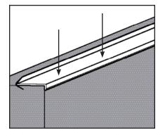
c. Press the DoorTop firmly onto the panel along the entire length. Close the door to confirm proper installation.
