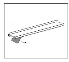
a. Remove the backing strip from attachment tape on underside of DoorTop
