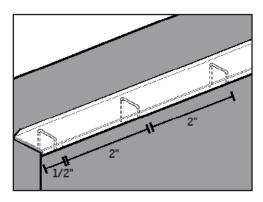
b. Attach the DoorTop to the top of the door panel using  $1/2" \times 1/2"$  staples. Position staples 1/2" from the end of the doortop and space them 2-4" apart. Close the door to confirm proper installation.
