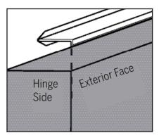
a. Orient the DoorTop with the door panel as shown above. Align the DoorTop flush to the edge of the hinge side.
