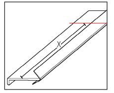
b. Measure and mark the same width (X) on the DoorTop, measuring from one end. Cut the DoorTop along this line.
