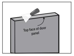
b. Remove any old residue or staples from the door panel's top face, using a putty knife or similar tool.
