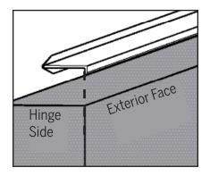
b. Align the end of the DoorTop seal flush to the edge of the hinge side along the outside of the door panel.
