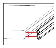
b. Using hand pressure (or a rubber mallet), fully insert the door bottom kerf legs into the panel slots, ensuring ends remain flush.
