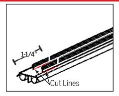
c. Cut the kerf legs, where they meet the door bottom until they are removed. Be sure to cut the kerf legs as close to the door bottom as possible to ensure a flat surface.
