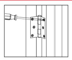
b. Reattach the hinges to the jamb with the screws previously removed. Confirm the door operates properly.
