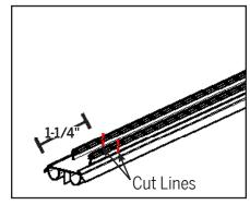
b. If the notch is less than 1-1/4", renotch the kerf legs. Measure 1-1/4" from the end of the door bottom and make a cut into the kerf legs.
