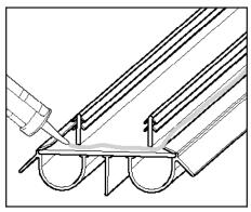
a. Apply exterior grade caulking along the edge of the door bottom that will be facing the exterior of the home. Thoroughly caulk each end of the door bottom.
