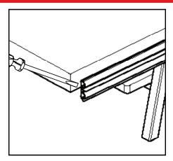
a. Remove the old door bottom from the door panel. Use a flathead screw driver to pry the end of the door bottom up.
