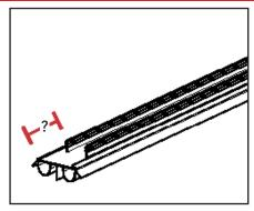
a. Measuring from the cut end of the door bottom, determine if the notch is greater or less than 1-1/4". If the notch is greater than 1-1/4", move to step 5.
