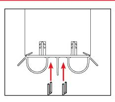
c. Complete insertion by moving along the length of the door bottom. Secure each end with a 1/2" x 1/2" light gauge staple. Wipe away excess caulking.
