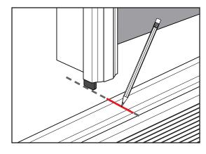
**a.** Close the inactive door and engage the upper and lower lock. Mark where the lock meets the sill cap. This will serve as a reference point to mount the strike plate.
