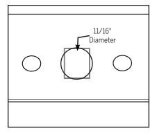
**c.** Drill into the header using an 11/16" diameter drill bit to create a space at least 1" deep.
