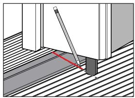
**a.** Close the inactive door and engage the upper and lower lock. Mark where the lock meets the sill cap or deck. This will serve as a reference point to mount the strike plate.
