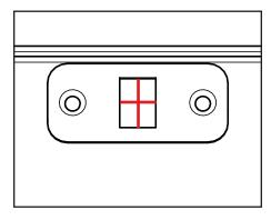
**a.** Using the marks you have made in Steps 4a and 4c, line up the strike plate on the header.
