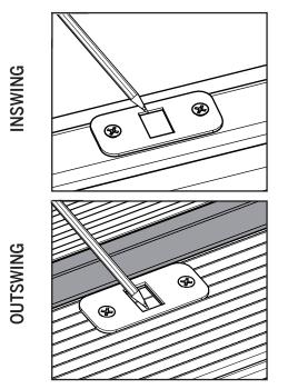
**a.** Trace the rectangular space of the strike plate with a pencil to use as a template to drill the holes.
