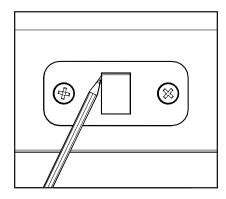
**a.** Trace the rectangular space of the strike plate with a pencil to use as a template to drill the hole.
