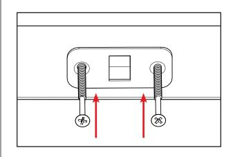
**a.** Return the strike plate to the exact position it was before (Step 5) and screw into place.
