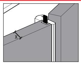
**b.** Measure the thickness of the door panel (X).
