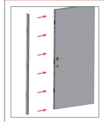
**a**. Install the routed astragal over the lock and onto the door panel.
