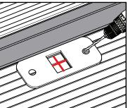
**b.** Spot drill the location of the screw holes.
