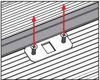
b. Unscrew and remove the strike plate.
