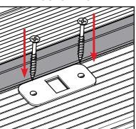
**a.** Return the strike plate to the exact position it was before (Step 9 & 10) and screw into place.
