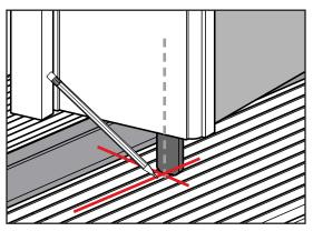
**b.** Close the door and mark the centerline of the door panel onto the sill deck.
