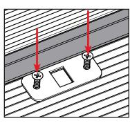
$\ensuremath{\textbf{c}}.$  Temporarily secure the plate to the sill using the 3/4" mounting screws.
