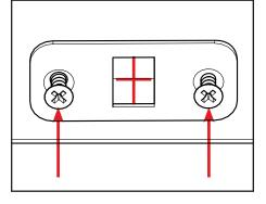
**c.**Temporarily secure the plate on the header using the 3/4" mounting screws.
