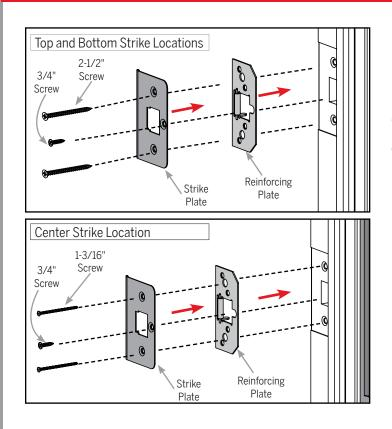
Align the three holes on the strike plate with the reinforcing plate and install on the astragal, ensuring the appropriate screws are used at each location.
