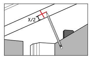
**c.** Divide this thickness (X) in half and mark that distance on the header. This will help you center the plate.
