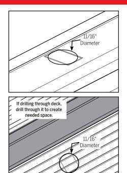
**c.** Drill into the sill cap or deck using an 11/16" diameter drill bit to create a space at least 1" deep.
