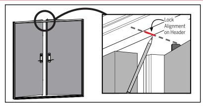
**a**. Close the inactive door and engage the lock. Mark the area where the lock will meet the header. This will serve as a reference point to mount the strike plate.
