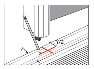
**b.** Measure the width of the sill cap (Y) and mark the center point (Y/2).
