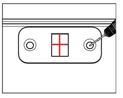
**b.** Spot drill the location for the screw holes.
