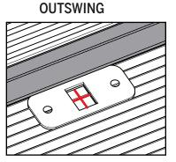
**a.** Using the marks you have made in Step 8, line up the strike plate on the sill cap or deck.
