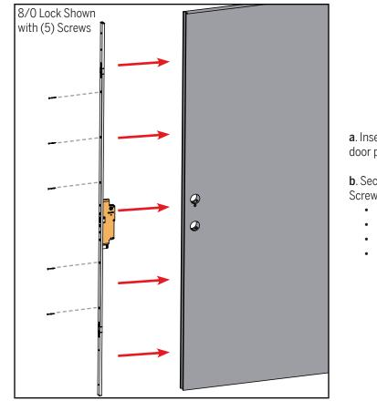
**a**. Insert the Trilennium 3020 Lock into the routed slot in the inactive door panel.
