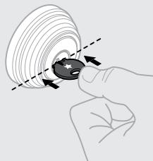
**Make sure new key (C) is FULLY inserted into lock.**
