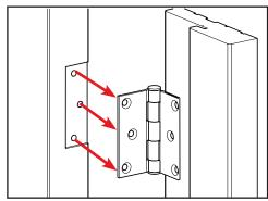
a. Realign the door panel with the hinges on the frame.
