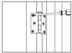
b. Reattach the hinges to the jamb with the screws. Confirm the door operates properly.
