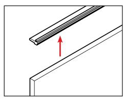
b. Remove the astragal from the door panel. Be sure to keep the fasteners to use when reinstalling.
