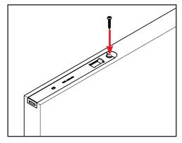
b. Screw the Magnum Bolt into the panel securely.
