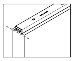
a. Align the retracted Magnum Bolt with the top or bottom of the door panel, depending on your desired location.
