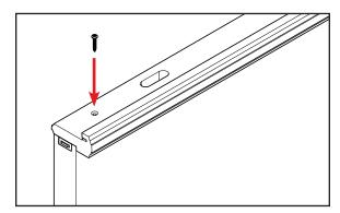
c. Secure the astragal through the Magnum Bolt to the door panel using a screw through the hole(s) you drilled into the astragal that align with the holes in the Magnum Bolt.
