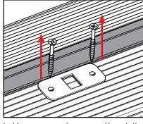
b. Unscrew and remove the strike plate.
