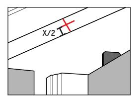
b. Divide this thickness (X) in half and mark that distance on the header. This will help you center the plate.
