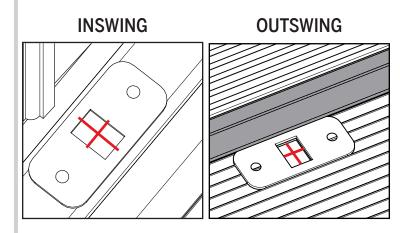
a. Using the marks you have made in Steps 7 and 8, line up the strike plate on the sill cap or deck.
