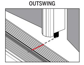
Close the inactive door and turn the lock to engage the upper and lower bolts. Mark where the lock meets the sill cap or deck. This will serve as a reference point to mount the strike plate.
