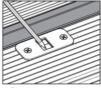
a. Trace the rectangular space of the strike plate with a pencil to use as a template to drill the holes.
