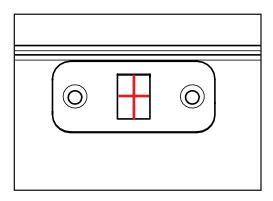
a. Using the marks from Steps 1 and 2, line up the strike plate on the header.
