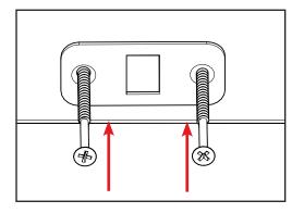
b. Spot drill the location of the screw holes. Once spot drilled, secure the plate into the header temporarily with the screws provided.
