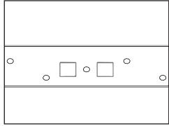
b. Unscrew and remove the strike plate.
