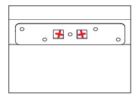
a. Using the marks you have made in Steps 1 and 2, line up the strike plate on the header.
