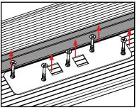
b. Unscrew and remove the strike plate.
