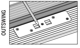
a. Trace the rectangular space of the strike plate with a pencil to use as a template to drill the holes.
