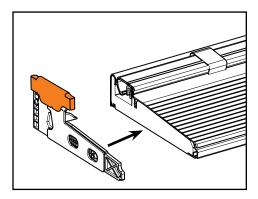
a. Place the Z-End Base<sup>TM</sup> against the end of the <u>uninstalled</u> sill as shown in image.
