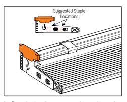
b. Staple the base onto the side in the locations shown. Repeat this on the other end of the sill with the other Z-End Base $^{\text{TM}}$ .
