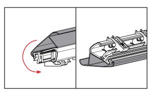
**a.** With the front hook still engaged, turn the cap over so the bottom of the spring-loaded bases are exposed.
