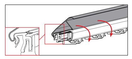
**a.** Starting at one end, engage the smaller hook of the cap cover with the shorter hook of the Z-AC cap. Press down along the length of the cap to ensure the cover securely fits into the front hook of the cap.
