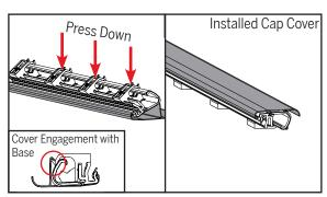
**b.** Press down on each base, compressing the cap, to connect the vertical hook to the catch on the center base.
