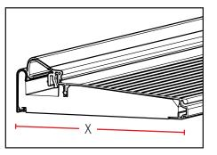
**a.** Measure the width of the sill (X) requiring the Z-End Base.
