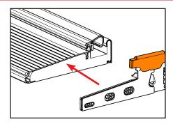
**a.** Place the sized Z-End Base against the end of the uninstalled sill as shown in the image.
