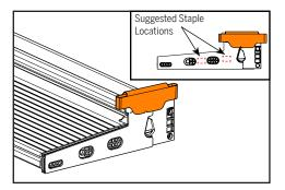
**b.** Staple the base onto the side in the locations shown. Repeat this on the other end of the sill with another Z-End Base.
