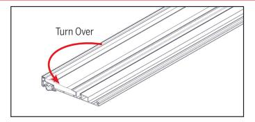
**a.** Turn the sill over, aluminum facing downward, on a covered flat surface. Using hand, press down on the sill to engage the lower clip.
