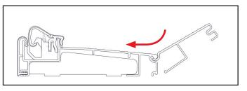
**a.** Align the hook of the extender into the top extender groove on the sill.
