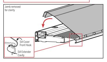
**a.** Engage the front hook of the sill cover into the sill extender cavity and rotate it over the deck and sill cap.
