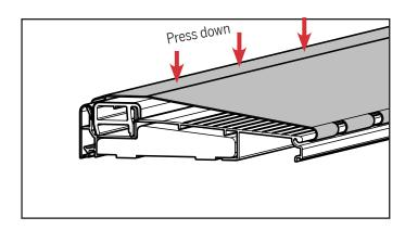
**b.** Press the sill cover down along the length of the sill cap to ensure it is securely attached.
