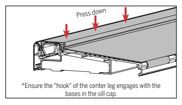
**b.** Press down on the sill cover along the sill length so that it is secure between the cap and the back of the sill.
