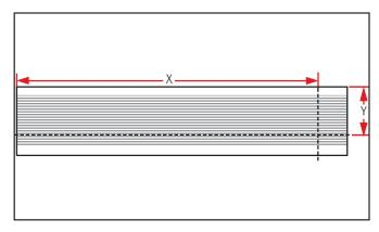
**b.** Cut the replacement sill deck to the measured width (unless 7-13/16" wide sill). Remove sharp edges from all areas.
