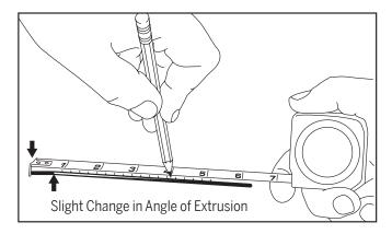
**a.** Measure and mark sill repair aluminum from the edge the arrows point to.
