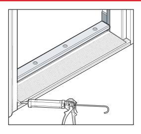
**a.** Caulk both ends of the replacement sill deck. Allow all caulk and adhesive to dry before stepping on sill.
