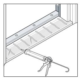
**a.** Apply construction adhesive (such as Liquid Nails) as rows along the surface of the existing sill.
