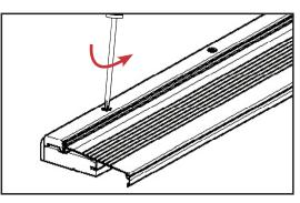
a. Remove the wood sill cap by gradually loosening the screws across the length of the sill. Remove and set aside
