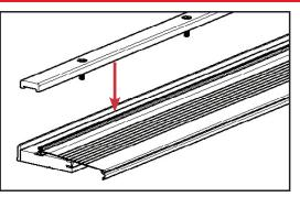
b. Replace the sill cap by screwing into place. Tighten the screws incrementally along the cap for a uniform reinstallation.
