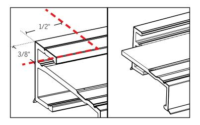
**a.** Notch the end of the sidelite seat by cutting the raised back and ensure a good fit against the jamb.
