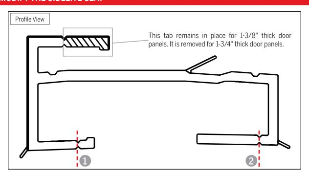
To convert the inswing sidelite seat into an outswing sidelite seat, identify the notches in the areas indicated in the image above at positions 1 and 2. Cut at these notches, along the length of the sidelite seat, and remove.
