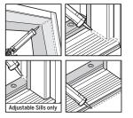
Door Sill Adjustment: Your Certified Powered By Endura<sup>™</sup> Door System incorporates an all-composite Z-Series Sill from Endura. The following steps should be taken at least one (1) time per year to ensure proper sealing and prevention of air and water infiltration (NOT APPLICABLE TO ARTICULATING AND OUTSWING CAPS):
