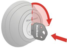
Insert functioning key & turn 1/4 turn clockwise
