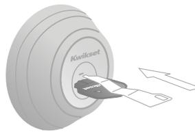
Insert & remove the SmartKey learn tool. Remove functioning key.
