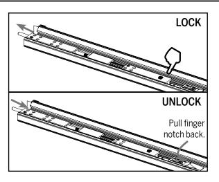
**f.** Confirm proper bolt operation by pushing the black button to engage the bolt and pulling back the finger notch to retract it.
