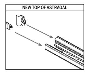
**a.** On what is now the top of the astragal, install the upper trim cap on the **wide side** and a tail cap on the **narrow side**.
