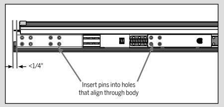
If the holes on the bolt do not align with the holes in the astragal body, adjust the location of the bolt sleeve and/or the push button housing to align the holes and then insert the orange securing pins. The bolt sleeve may be up to 1/4" inset from the end of the astragal.
