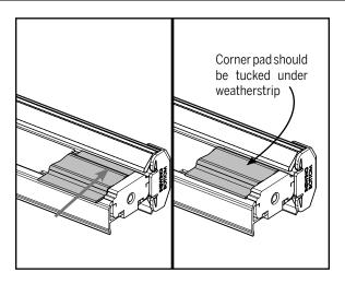
**e.** Once the lower bolt is installed, realign the Simple Solution Corner Pad under the weatherstrip.
