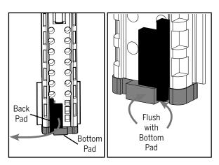
**b.** Before replacing the lower bolt, remove the existing back pad and place a new one mirroring the original pad.
