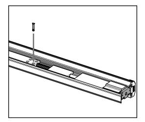
**d.** Insert the orange securing pin into the hole on the bolt sleeve that aligns with the hole in the astragal body. If holes do not align, see gray box on Page 3 to align holes.
