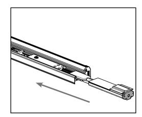
**c.** With the bolt in the unlocked position, slide the lower bolt back into the astragal.
