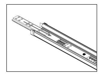
**b.** Return the **retracted** upper bolt by sliding it back into the astragal body until the end of the bolt sleeve is flush with the end of the astragal. If a tail cap is present, the bolt should be flush with the tail cap.
