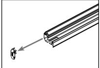
b. Reverse the astragal: Rotate the astragal so the upper and lower ends are reversed.
