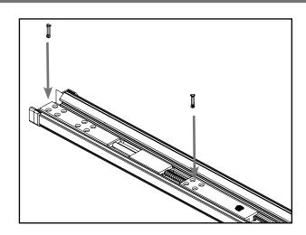
**c.** Insert the two orange securing pins into the bolt in the holes that align with the holes in the astragal body. (See below if holes are not aligned.)
