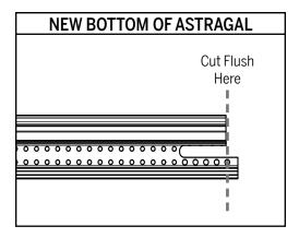
**a.** Using a chop saw, cut the **narrow side** of the astragal, so it is flush with the wide side.
