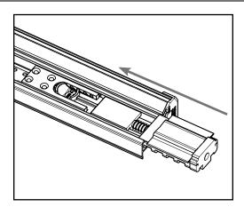
c. With the bolt in the unlocked position, slide the lower bolt back into the astragal.
