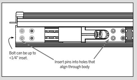
If the holes on the bolt do not align with the holes in the astragal body, adjust the location of the bolt sleeve and/or the finger notch housing to align the holes and then insert the orange securing pins. The bolt sleeve may be up to 1/4" inset from the end of the astragal.
