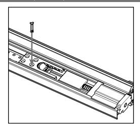
**d.** Insert the orange securing pin into the hole on the bolt sleeve that aligns with the hole in the astragal body. If holes do not align, see gray box on Page 3 to align holes.
