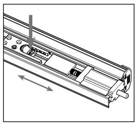
**f.** Confirm proper bolt operation by pressing down on the finger notch to pull and retract it.
