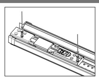
**c.** Insert the two orange securing pins into the bolt in the holes that align with the holes in the astragal body. (See below if holes are not aligned.)
