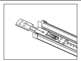
**b.** Return the **retracted** upper bolt by sliding back into the astragal body until the end of the bolt sleeve is flush with the end of the astragal. If a tail cap is present, the bolt should be flush with the tail cap.
