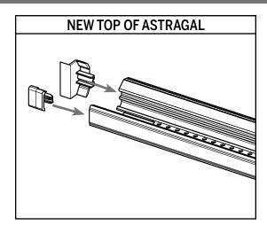
**a.** On what is now the top of the astragal, install the upper trim cap on the **wide side** and a tail cap on the **narrow side**.
