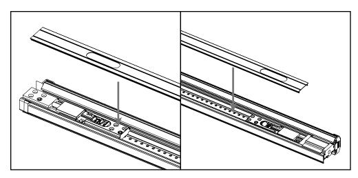
**a.** Reinstall the trim strip onto the astragal. The trim strip with the larger space between the notch and edge will be for the top of the astragal.
