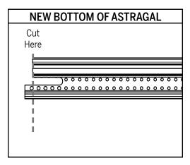
**a.** Using a chop saw, cut the **narrow side** of the astragal, so it is flush with the wide side.
