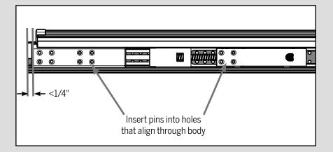
If the holes on the bolt do not align with the holes in the astragal body, adjust the location of the bolt sleeve and/or the push button housing to align the holes and then insert the orange securing pins. The bolt sleeve may be up to 1/4" inset from the end of the astragal.
