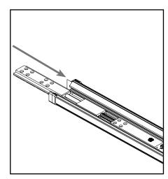
**c.** Return the upper bolt by sliding it back into the astragal body until the end of the bolt sleeve is flush with the end of the astragal.
