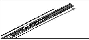
**b. Remove strike support:** Remove the screw that secures the strike support and slide the strike support out of the astragal to remove.
