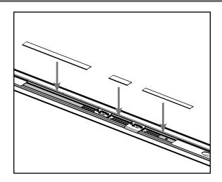
**a.** Reinstall the trim strips into the astragal. The wider trim strip with the larger space between the notch and edge will be for the top of the astragal. The narrow trim strip will be installed into the strike support.
