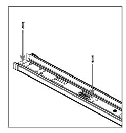
**d.** Insert the two orange securing pins into the bolt in the holes that align with the holes in the astragal body (See next page if holes are not aligned).
