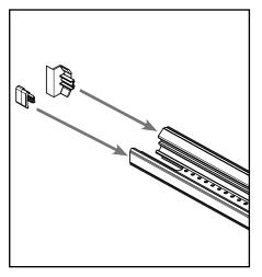
**b.** On what is now the top of the astragal, install the upper trim cap on the **wide side** and a tail cap on the **narrow side**.
