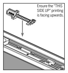
**b**. Reinstall the lower bolt head back into the drive rods.
