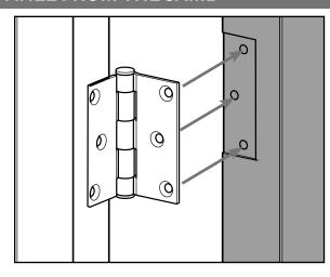
**b**. Remove screws and detach the inactive door panel from the hinges.
