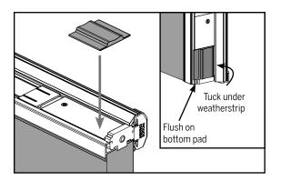
**d**. Install a new corner pad (purchased separately). Corner pads should be installed flush against the bottom pad and tucked under the weatherstrip.
