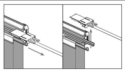
**d**. Slide out the lower metal drive rods and remove the shoot bolt.
