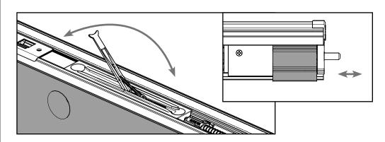
**a.** Operate the flip lever and ensure the bolt sleeve and pins move between engaged and disengaged positions.
