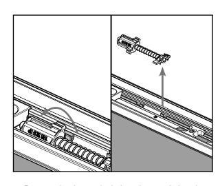
**c.** Rotate the lower bolt head out of the drive rods and remove that assembly from the astragal body.
