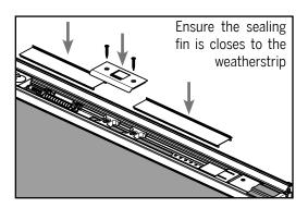
**a**. Reinstall the lower strike plate assembly and trim strips previously removed from the astragal body.
