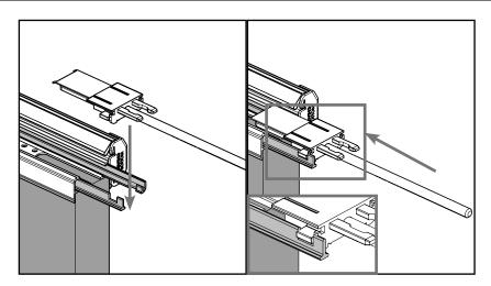
**a**. Return the shoot bolt so its engagement head notches securely into the grooves on the metal drive rods. Slide the rods back in place.
