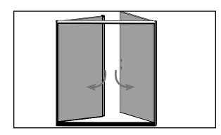
**c.** Close the inactive door and lock the bolts to confirm proper operation.
