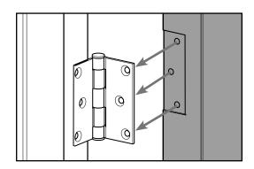
**b**. Reinstall the inactive door panel by screwing the door panel back to the hinges.
