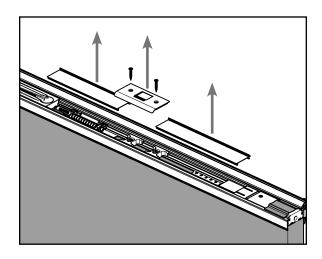
**a**. Remove the bottom two pieces of trim strip and the lower strike plate assembly. Set aside.
