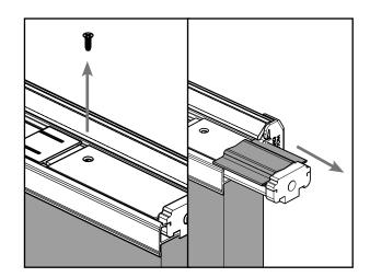
**b.** Remove the screw securing the lower bolt sleeve. Slide the bolt sleeve out of the astragal body.
