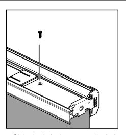
**c**. Slide the bolt sleeve onto the bolt and secure by reinstalling the screw.
