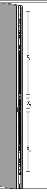
**a.** Measure the distance from the top of the astragal body to the deadbolt plate  $(X_1)$ , between the deadbolt plate and the strike plate and between the strike plate  $(X_2)$  and the bolt sleeve on the lower bolt  $(X_3)$ . Ensure the bolts are in the retracted position to get an accurate measurement.
