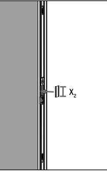
**e.** Cut the remaining trim strip to match the length  $(X_2)$  measured in Step 2 between the deadbolt and strike plates and install.
