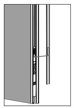
**c.** Align the second oblong cutout of the trim strip with the finger grip on the lower bolt.
