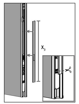
**d.** Cut the trim strip to match the length  $(X_3)$  measured in Step 1 and install on the lower half of the astragal. Cut any overhang past the lower bolt sleeve.
