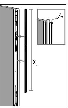
**b.** Cut the trim strip to the size  $(X_1)$  measured in Step 1 and install on the upper half of the astragal. If there is any overhang past the top of the upper bolt, cut the trim strip to fit flush with the end of the astragal bolt,
