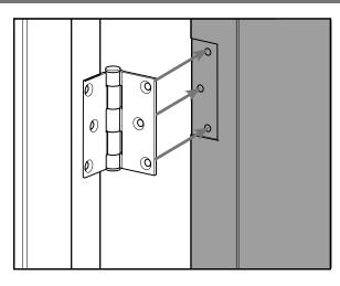
**b**. Remove the screws securing the inactive door to the hinges.
