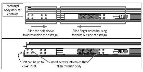
**b**. If the holes on the bolt do not align with the holes in the astragal body, adjust the location of the bolt sleeve and/or finger notch housing to align the holes. The bolt sleeve may be up to 1/4" inset from the end of the astragal.
