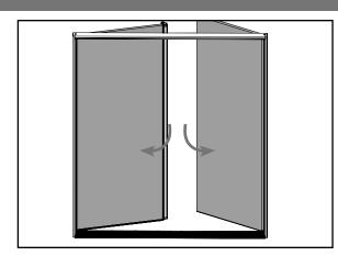
**c.** Close the inactive door and lock the bolts to ensure the bolts contact the header and sill receivers properly.
