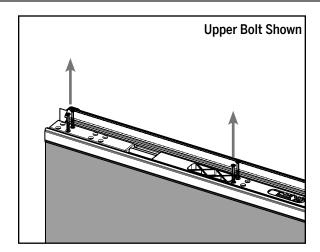
**b.** Remove the screws securing the bolt into the astragal body and door panel and set aside.
