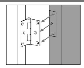
**b**. Reinstall the inactive door panel by screwing the door panel back to the hinges.
