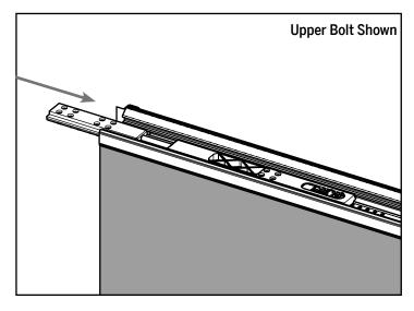
**a**. Slide the new bolt into the astragal body until the end of the bolt sleeve is flush with the end of the astragal.
