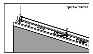
**c**. With holes aligned on the bolt sleeve and the finger notch housing, insert the screws previously removed through the holes and tighten.
