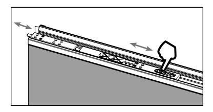
**a**. To check bolt operation, press down on the finger notch and slide the bolt out towards the end of the astragal. To unlock the bolt, press down and slide back.
