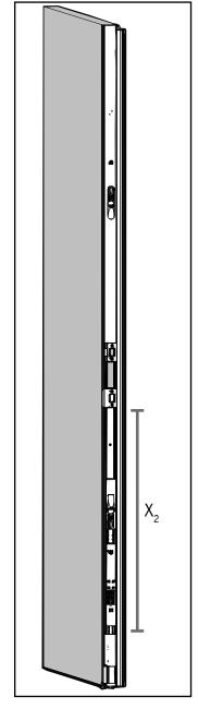
**a.** Measure and note the distance from the strike plate to the bolt sleeve on the lower bolt  $(X_2)$ .
