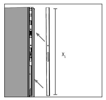
**c.** Cut the trim strip to size measured in Step 1a. Install sized trim strip onto the astragal body.
