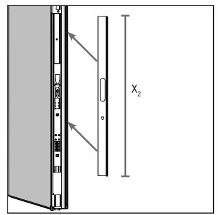
**c.** Cut the trim strip according to the measurement taken in Step 2a. Ensure the side with the sealing fin is on the same side as the weatherstrip. Install sized trim strip onto the astragal body.
