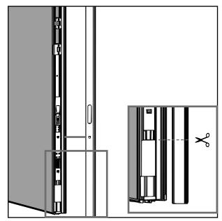
**b.** Align the D-shaped cutout on the trim strip with the push button on the lower bolt. Cut any overhang past the lower bolt sleeve.
