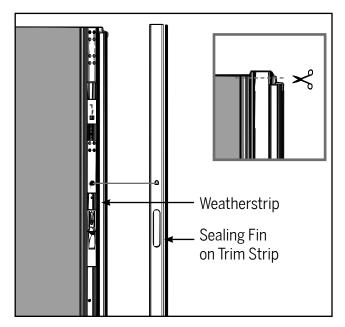
**b.** Align the D-shaped cutout on the trim strip with the push button on the upper bolt. If there is any overhang past the top of the upper bolt, cut the trim strip to fit flush with the end of the astragal. Ensure the side with the sealing fin is on the same side as the weatherstrip.
