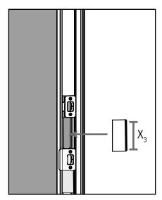
**b.** Cut the remaining trim strip to match this length and install into the astragal. Ensure the side with the sealing fin is on the same side as the weatherstrip.
