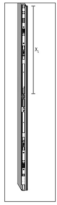
**a.** Measure and note the distance from the top of the deadbolt plate to the top of the astragal  $(X_1)$ .
