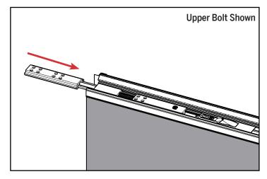
**a**. Slide the new bolt into the astragal body until the end of the bolt sleeve is flush with the end of the astragal.
