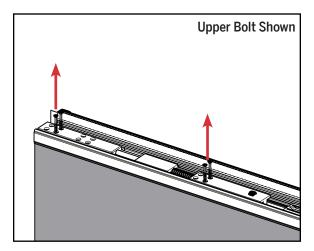
**b.** Remove the screws securing the flush bolt into the astragal body and door panel and set aside.
