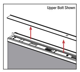
**a**. Remove the trim strip covering the bolt being replaced and set aside.
