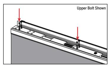
**c**. With holes aligned on the bolt sleeve and the push button housing, insert the screws previously removed through the holes and tighten.
