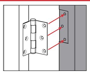
**b**. Remove the screws securing the inactive door to the hinges.
