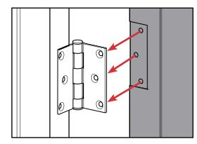
**b**. Reinstall the inactive door panel by screwing the door panel back to the hinges.
