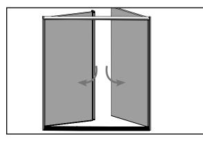
**c.** Close the inactive door and lock the bolts to confirm proper operation.
