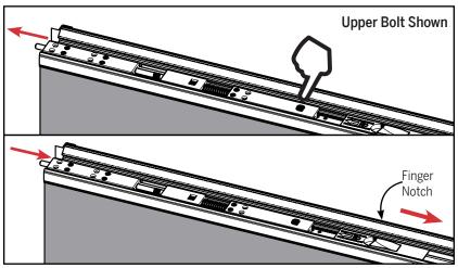
**a**. Press the push button on the new bolt to ensure the bolt was properly installed. Retract the bolt by pulling the finger notch back.
