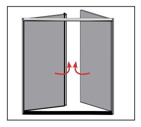
**a**. Open both door panels to access the hinges of the inactive door panel.
