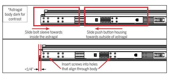
**b**. If the holes on the bolt do not align with the holes in the astragal body, adjust the location of the bolt sleeve and/or push button housing to align the holes. The bolt sleeve may be up to 1/4" inset from the end of the astragal.
