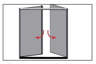
**c.** Close the inactive door and lock the bolts to confirm proper operation.
