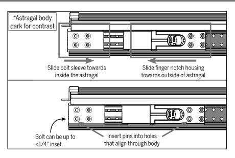
**b**. If the holes on the bolt do not align with the holes in the astragal body, adjust the location of the bolt sleeve and/or finger notch housing to align the holes. The bolt sleeve may be up to 1/4" inset from the end of the astragal.
