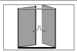
**c.** Close the inactive door and lock the bolts to ensure the bolts contact the header and sill receivers properly.
