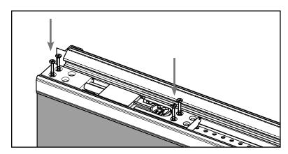
**c**. Insert screws into the holes on the bolt sleeve and finger notch housing that are aligned with the holes in the astragal body. Tighten so the surface of the screw is just flush with the surface of the bolt.
