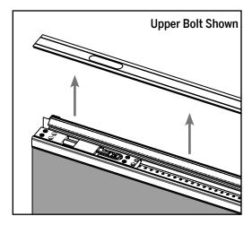
**a**. Remove the trim strip covering the bolt being replaced.
