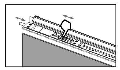
**a**. To check bolt operation, press down on the finger notch and push the bolt out towards the end of the astragal. To unlock the bolt, press down and slide back.
