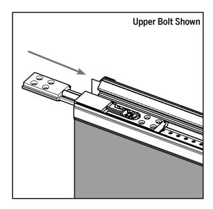
**a**. Slide the new bolt into the astragal body until the end of the bolt sleeve is flush with the end of the astragal.
