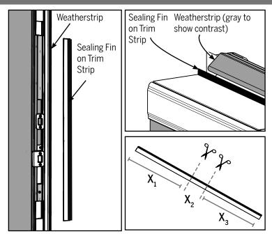
Orient the trim strip against the astragal so that the side with the sealing fin is close to the weatherstrip. Cut the trim strip into sizes matching the distances measured in Step 1.
