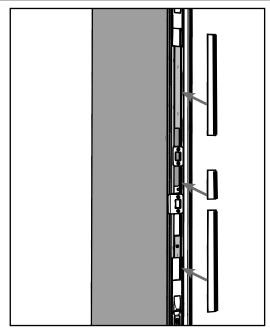
Install each piece of the trim strip onto the strike support, ensuring the side with the sealing fin is close to the weatherstrip.
