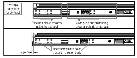
**b**. If the holes on the bolt do not align with the holes in the astragal body, adjust the location of the bolt sleeve and/or push button housing to align the holes. The bolt sleeve may be up to 1/4" inset from the end of the astragal.
