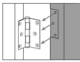
**b**. Reinstall the inactive door panel by screwing the door panel back to the hinges.
