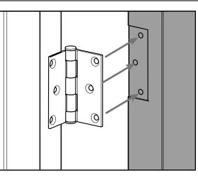
**b**. Remove the screws securing the inactive door to the hinges.
