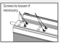
**For Upper Bolt Only:** If retracting the bolt is tight, loosen the screws on the upper bolt
