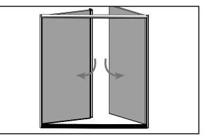
**c.** Close the inactive door and lock the bolts to ensure the bolts contact the header and sill receivers properly.
