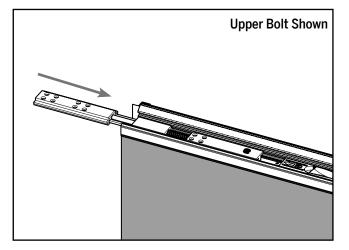
**a**. Slide the new bolt into the astragal body until the end of the bolt sleeve is flush with the end of the astragal.
