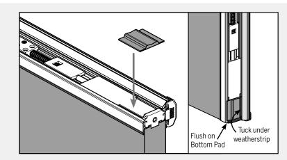
**NOTE:** If replacing the lower bolt, install a new corner pad (purchased separately) at this step.
