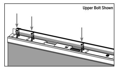
**c**. Insert screws into the holes in the bolt sleeve and the push button housing that align with the holes in the astragal body. Tighten until the screws are just flush with the surface of the bolt.
