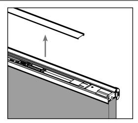
**a**. Remove the trim strip covering the lower bolt and set aside.
