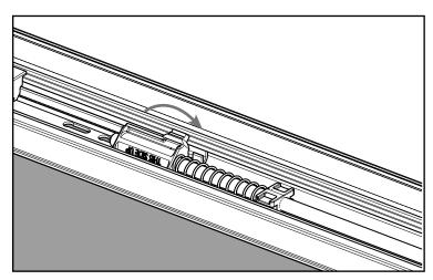
**b**. Check that the bolt head is in the correct orientation. "THIS SIDE UP" printing should be visible. Rotate the bolt head into the upper drive channel.
