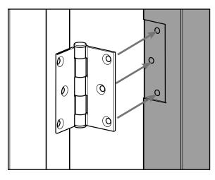
**b**. Remove screws and detach the inactive door from the hinges.
