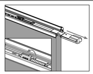
**b.** Rotate the bolt head out of the drive channel to freely slide the bolt out of the astragal. Discard the bolt.
