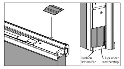
**c.** Install a new corner pad (purchased separately). Corner pads should be installed flush against the bottom pad and tucked under the weatherstrip.
