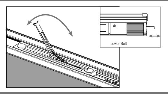
**a.** Operate the flip lever and ensure the lower bolt is properly engaged. If the lower bolt does not freely move, the lever may need to be cycled several times.
