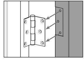
**b**. Reinstall the inactive door panel by screwing the door panel back to the hinges.
