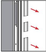
**a.** Remove damaged or old strike plates and strike retainers and discard. If necessary, remove the trim strip and set aside.
