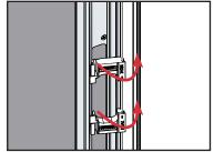
**d.** Break retainer in half using the bend lines. Insert the two pieces of the retainer to the astragal by pressing the tabs to snap into place.
