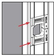
**b.** Press lightly against the two tabs, and snap the retainer into place.
