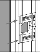
**b.** Press lightly against the two tabs, and snap the retainer into place.
