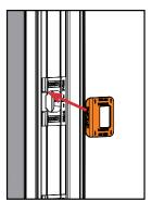
**c.** Install the strike plates onto the strike retainers. Dummy plates included in the kit can be pressed into the retainers. Alternately, final metal hardware may be installed
