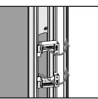
**d.** Break retainer in half using the bend lines. Insert the two pieces of the retainer to the astragal by pressing the tabs to snap into place.
