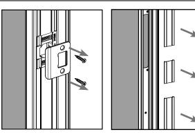
**a.** Remove damaged or old strike plates and strike retainers and discard. If necessary, remove the trim strip and set aside.
