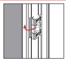
**a.** Angle the strike retainer and rotate it into the astragal body.
