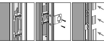
**e.** Adjust the location of the two pieces of the retainer and install the new hardware. Replace trim strip if it was removed.
