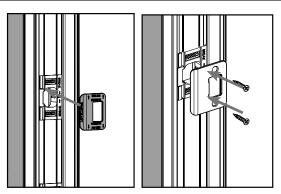
**c.** Install the strike plates onto the strike retainers. Dummy plates included in the kit can be pressed into the retainers. Alternately, final metal hardware may be installed.
