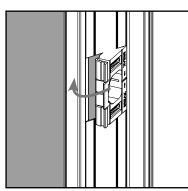
**a.** Angle the strike retainer and rotate it into the astragal body.
