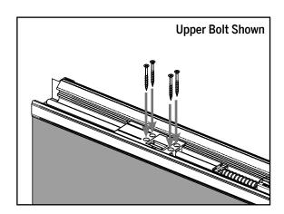
**d**. Reinstall the four screws surrounding the lock pawl.
