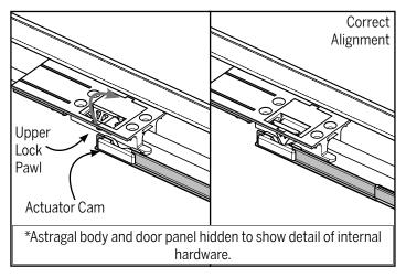
**c.** Adjust the T-bar to align the actuator cam with the lock pawl. Lift the upper lock pawl and slide the actuator cam under it, allowing it to mate with the lock pawl.
