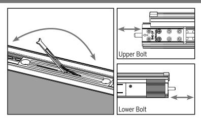
**a.** Operate the flip lever and ensure the bolt sleeve and pins move between engaged and disengaged positions.
