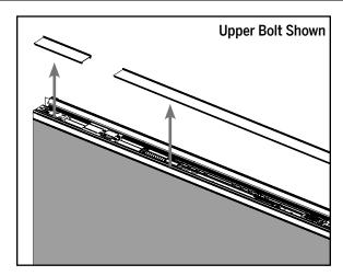
**a**. Remove the trim strip(s) covering the bolt being replaced and set aside.
