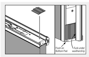
**NOTE:** If replacing the lower bolt, install a new corner pad (purchased separately) at this step.
