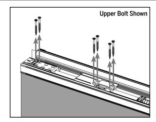
**b.** Remove the 6 screws from the upper bolt (4 around lock pawl and 2 from bolt sleeve) and set aside.
