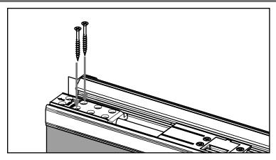
**g**. With the holes aligned on the bolt sleeve, insert the two screws previously removed through the hole and tighten.
