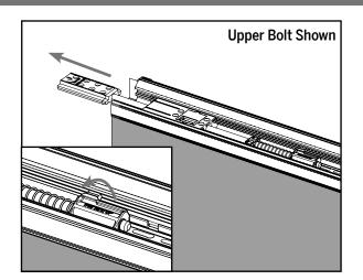
**c.** Rotate the bolt head out of the drive channel and slide the bolt and bolt sleeve out of the astragal. Discard the old bolt.
