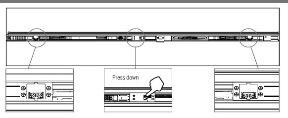
**b.** Operate the deadbolt actuator, ensuring the upper and lower lock pawls move between engaged and disengaged positions. Check that there is no binding between the lock pawls when the deadbolt actuator is fully depressed and that the pawls move at the same time.
