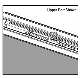
**b**. Check that the bolt head is in the correct orientation. "THIS SIDE UP" printing should be visible. Rotate the bolt head into the upper drive channel.
