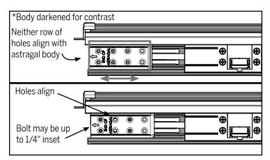
**f.** Adjust the bolt sleeve until the first or second row of holes aligns with the holes in the astragal body.
