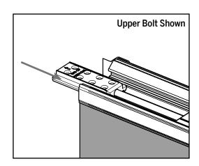
**e**. Slide the bolt sleeve into the astragal body, allowing it to slide along the bolt.
