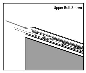
**a**. Slide the new bolt into the astragal body until the end of the bolt is flush with the end of the astragal.
